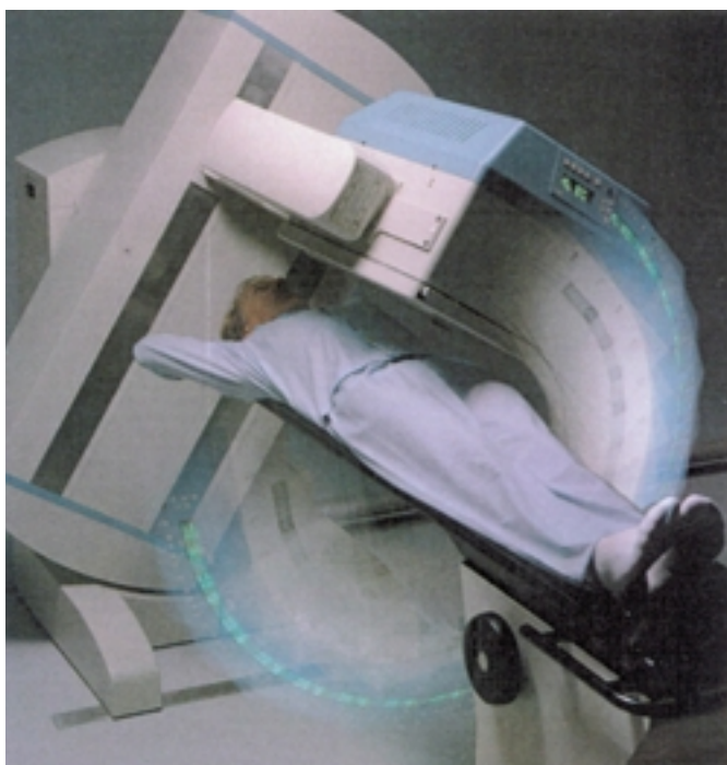
Figure 8.1 Example of a single detector gamma camera and its movement during SPECT acquisitions. Image supplied by ADAC Medical Systems.
