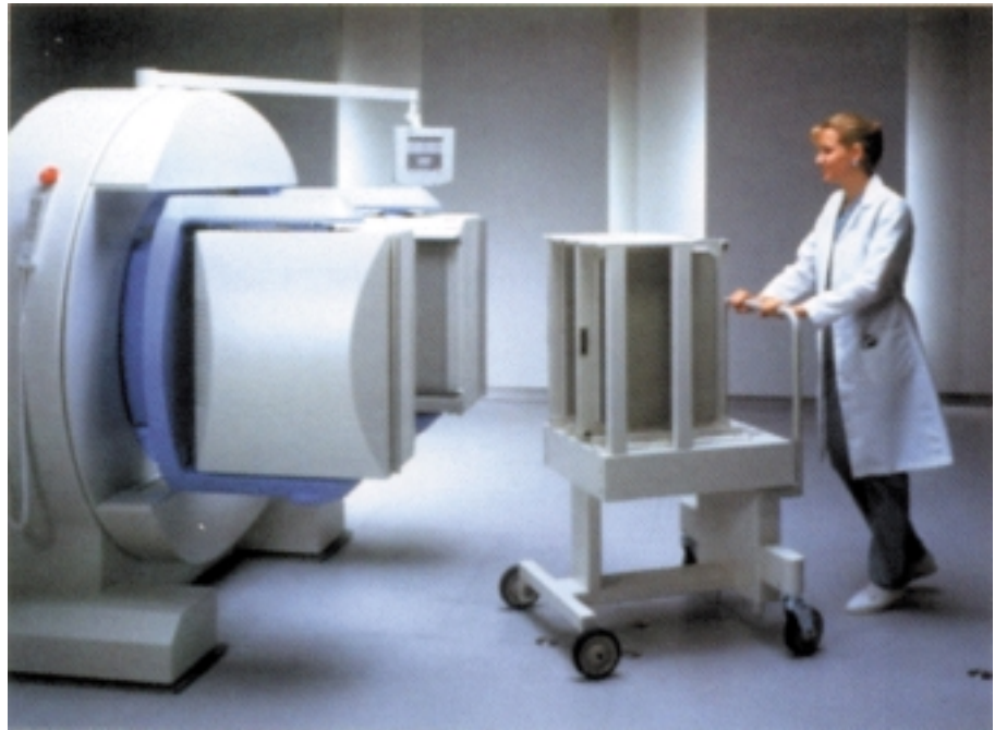
Figure 8.2 Example of a dual detector gamma camera. Image supplied by Siemens Medical Solutions.
